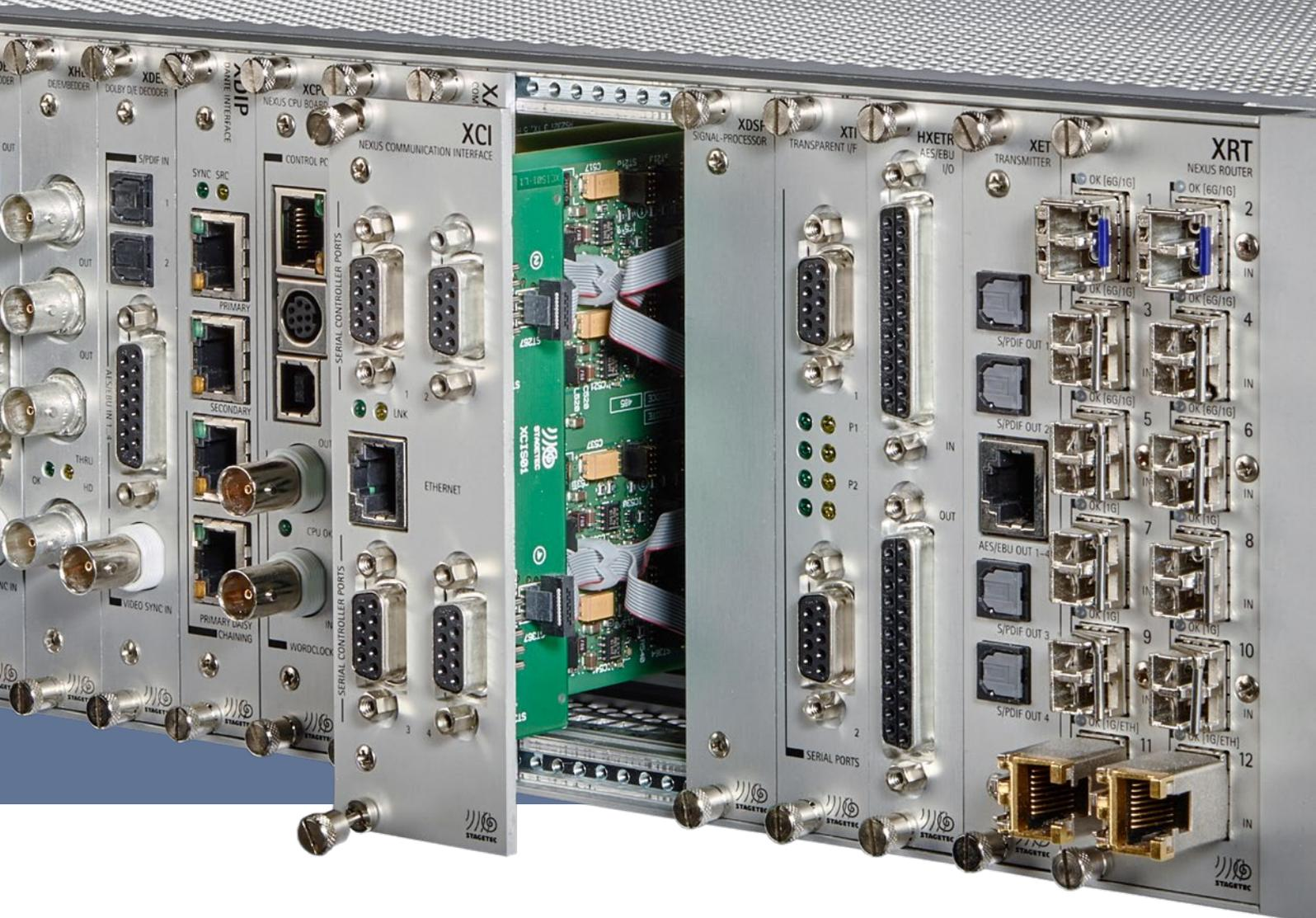
**Combined version with BNC input, BNC output and LC optical connection**
