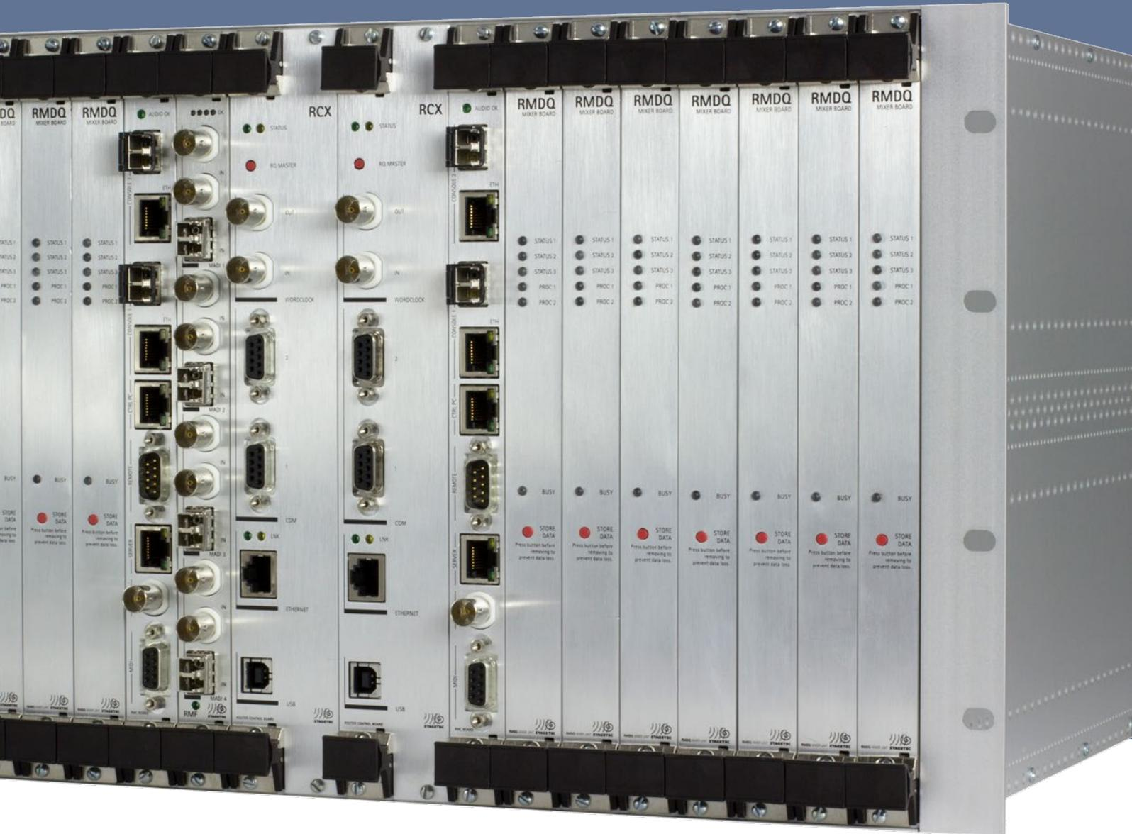
event of a switchover or failure of a sync source, so that there are never dropouts or crackles in the audio. In conjunction with a cleverly defined sync hierarchy, the board offers a wide range of connection options that ensure that the NEXUS system synchronizes itself to the current application, stabilizes this sync and passes it on to other systems.
